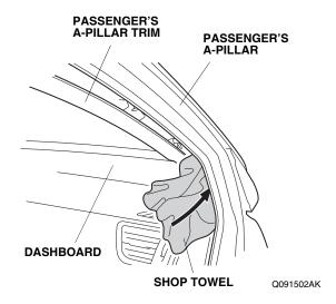
Remove the passenger's A-pillar trim from the upper clip (unplug the vehicle connector, if equipped).
