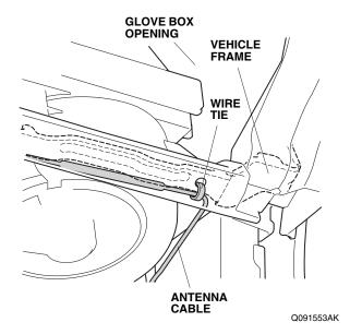
48. Bundle the antenna cable, and secure it to the vehicle harness with one wire tie.
