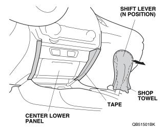
18. Remove the center lower panel (two self-tapping screws, four clips, and unplug the vehicle connectors, if equipped).
