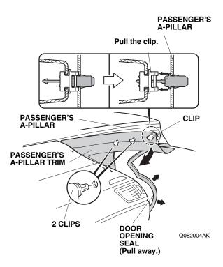
7. Pull out the passenger's A-pillar trim to release the clips.
